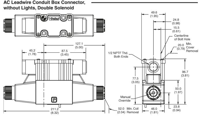
Note: 22.0 mm (0.87") from bottom of bolt hole counterbore to bottom of valve.
